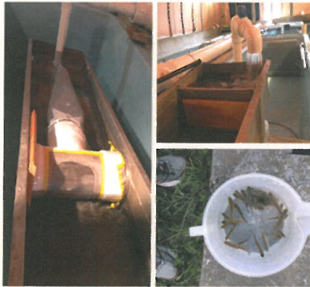
Left: Sloped raceway with drift net sampler positioned for sample collection. Note how flow has extended conical net. Top Right: Small holding pen below well water tap at top of sloped raceway. Bottom Right: Bucket showing ~60 rainbow trout used for biomass in experiment. 1 fry weighed ~1.3g.
