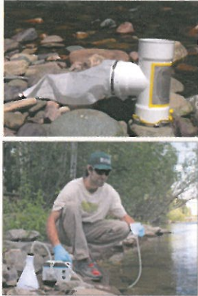
Top: Drift net with fine mesh used to sample 1000s of liters of water. Bottom: Typical filter sampler for small volume water samples (<5L).
